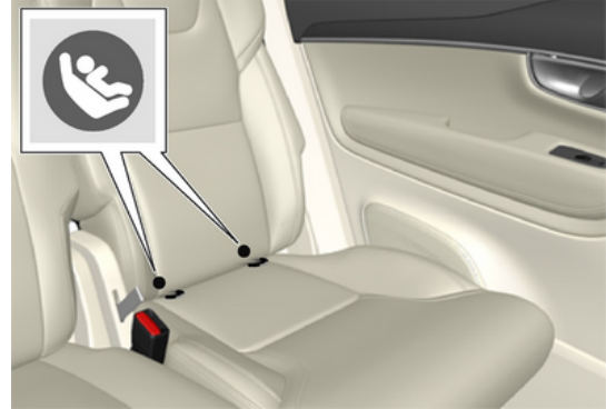
Image from ISOFIX/LATCH lower anchors | Attachment points for child seats | SaFety | XC90 2021 Early | Volvo Support. (volvocars.com)
